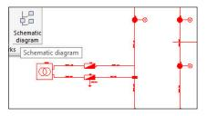
The generation of structural diagrams of networks starting from the power source to the final object. The functionality can be used to quickly generate a drawing of the structural diagram of a proposed network. The diagram contains the topology of the proposed network
